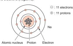
When two materials come into close contact, negative electrons move freely from molecule to molecule between the two.
