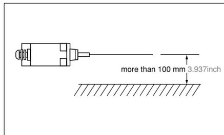
**3) Distance between antennas used in parallel**
