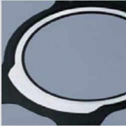
Removal of coating film from gasket
