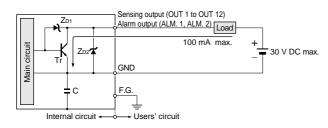
Symbols ... Z<sub>D1</sub>, Z<sub>D2</sub>: Surge absorption zener diode Tr: NPN output transistor C: Capacitor (1,000 pF)
