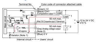
Notes: 1) As for the aluminum body type, varistor (clamping voltage approx. 40 V) is connected between the internal power circuit and the metal body to prevent breakdown of the sensor. Connect the metal body to +V of power supply or to frame ground (F.G.) of a device that is connected to 0 V. High potential and insulation resistance tests between the internal power circuit and the metal body must not be done.
