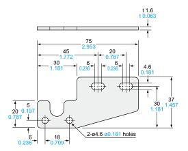
Material: Cold rolled carbon steel (SPCC) (Uni-chrome plated)
