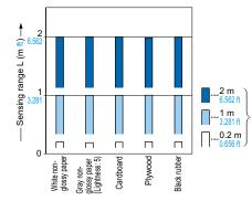
These bars indicate the sensing range with respective objects when the distance adjuster is set at the sensing range of 2 m 6.562 ft, 1 m 3.281 ft and 0.2 m 0.656 ft long, each, with white non-glossy paper.
