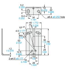
Material: Cold rolled carbon steel (SPCC) Two M4 (length 25 mm 0.984 in) screws with washers and two M4 nuts are attached.
