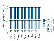
These bars indicate the sensing range with the respective colors when the distance adjuster is set at the sensing range of 2 m 6.562 ft, 1 m 3.281 ft and 0.2 m 0.656 ft long, each, with white color.
