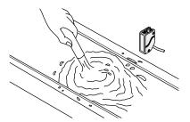
Note: If water splashes on the sensor during sensing operation, it may sense water as an object.
