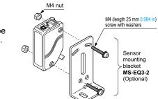
Care must be taken regarding the sensor mounting direction with respect to the object's direction of movement.
