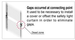
"ZERO" dead zone when using L-shaped mounting
