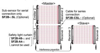
\* Set the frequency selection switches (for both emitter and receiver) to "1" at the master units, and set them to "2" at the slave units.
