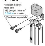
Attaches to top of safety light curtain. Tighten together the mounting bracket provided with the safety light curtain (MS-SF2B-1/4/5) and the mounting bracket of SF-IND-2.
