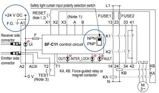
Notes: 1) The above diagram is when using manual reset. If automatic reset is used, disconnect the lead from X2 and connect it to X3. In this case, a reset (RESET) button is not needed.
