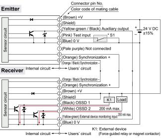
Note: Unused wires must be insulated to ensure that they do not come into contact with wires already in use.
