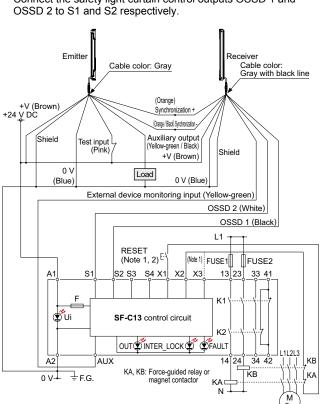
Notes: 1) The left diagram is when using manual reset. If automatic reset is used, disconnect the lead from X2 and connect it to X3. In this case, a reset (RESET) button is not needed.
