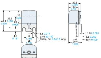
Material: Bracket ··· Cold rolled carbon steel (SPCC)(Black chromate)
