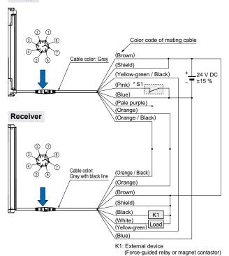
Note: Unused wires must be insulated to ensure that they do not come into contact with wires already in use.
