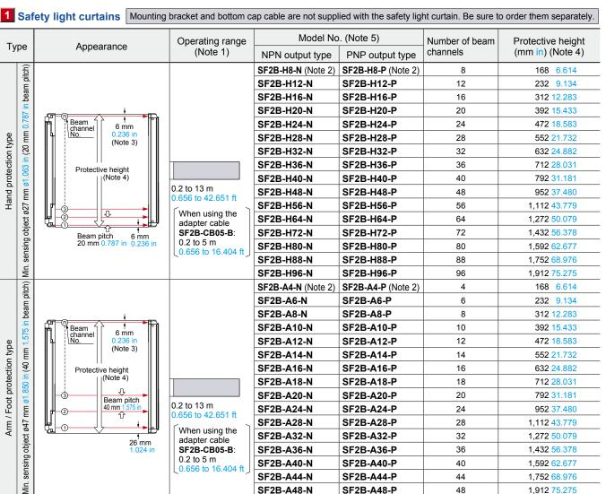
Notes: 1) The "operating range" is the possible setting distance between the emitter and the receiver
