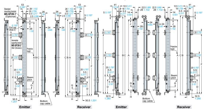
Notes: 1) The MS-SF2B-2 intermediate supporting bracket is provided as an accessory with this product. The number of accessories provided varies depending on the product. 2) An end cap (connector for series connection) is not provided for the SF2B-H8(SL)(-□) and SF2B-A4(SL)(-□).
