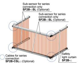
Hand protection type and Arm / Foot protection type can be used together.
