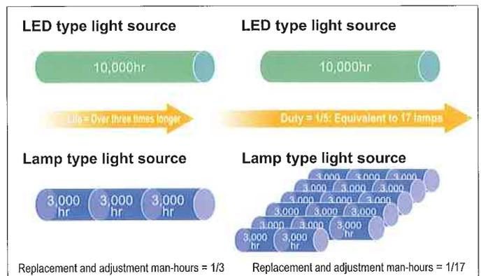
\* The 10,000-hour LED life is an estimate based on use of the head at 25°C and a UV intensity over 70% the initial value.
