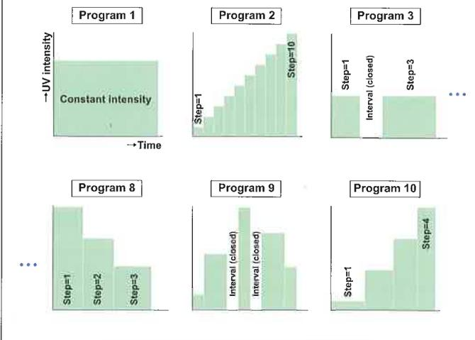
The irradiation pattern programming function allows changes in the irradiation intensity in accordance with the irradiation time.
