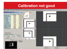
Auto calibration result: Vertical placement different from actual positional relationship
