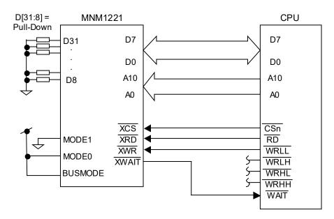
Note: For pull-down resistor for unused data-bus, about 10 k Ohm is recommended. The above figure shows an example of CPU with byte-unit address bus
