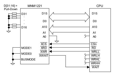
Note: Approximately 10 k Ohm is suitable for the pull-down registers on D[31:16]. The above figure shows an example of CPU with byte-unit address bus.
