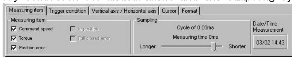
“Measurement items”: You can measure any of “Command speed” , “Torque” and “Position error” even at the same time.
