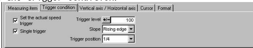
“Set the trigger of actual speed”: It is valid with check.
