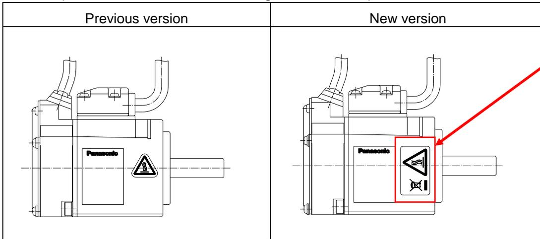
Recycling symbol is added to the high temperature caution mark, and the direction of the high temperature caution label is changed.
