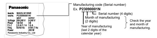
The manufacturing code (serial number) shown on the label attached to the front surface of the package box follows the following rule.
