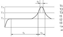
T1 = 150 to 180°C T2 = 230°C T3 = 240 to 250°C\* t1 = 60 to 120 s t2 = Within 30 s t3 = Within 10 s \*240 to 245°C for SON, VSSOP and TSON package
