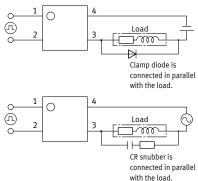
2) When Clamp diode or CR Snubber is used in the circuit, the spike voltages from the load are limited. But the longer wire may become the inductance and cause the spike voltage. Keep the wire as short as possible.
