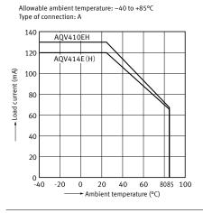
1-2.Load current vs. ambient temperature characteristics
