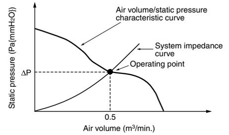
The intersection of the air volume/static pressure characteristic curve with the system impedance curve is called the operating point. This shows the condition with the fan motor operating.
