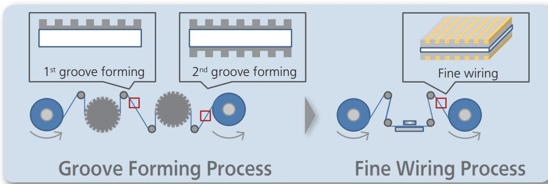
[High Aspect Ratio Wiring Line Forming] Realizes both low resistance & high transmissivity by fine and deep wire forming
