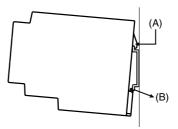
When dismounting the PM5S pull out portion (C) with a flatblade screwdriver and remove the Timer from the mounting track.
