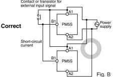
The PM5S series is provided with a transformer less power supply system.
