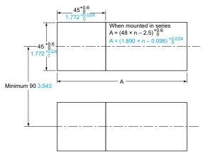
Note: The panel thickness should be 1 to 5 mm 0.039 to 0.197 in.
