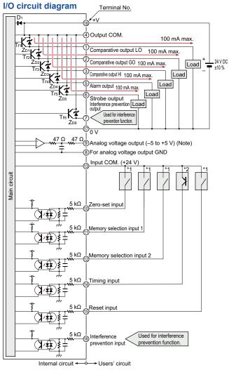
Note: Devices connected to the analog voltage output must have an input impedance set at 1  $\mbox{M}\Omega$  or more.
