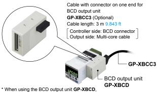
\* When using the BCD output unit GP-XBCD, the analog voltage output of a controller becomes invalid.
