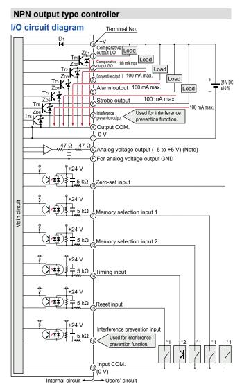
Note: Devices connected to the analog voltage output must have an input impedance set at 1  $\mbox{M}\Omega$  or more.
