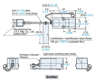
Note: IEC / JIS conforming products do not contain light beam shielding plate, or certification/identification label.
