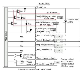
Symbols ... D: Reverse supply polarity protection diode Zo1, Zo2, Zo3: Surge absorption zener diode Tr1, Tr2, Tr3: PNP output transistor
