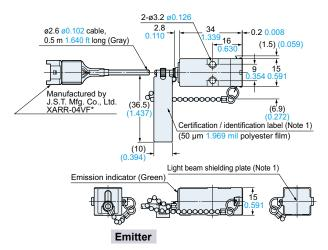
Notes: 1) IEC / JIS conforming products do not contain light beam shielding plate, or certification / identification label.
