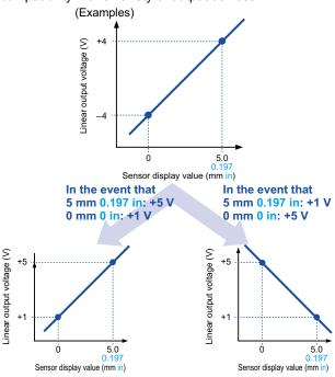
The linear output must be set by determining output values (maximum; current: 0 to 23.5 mA / voltage: ±5.5 V) at two different points, for the arbitrary display value.
