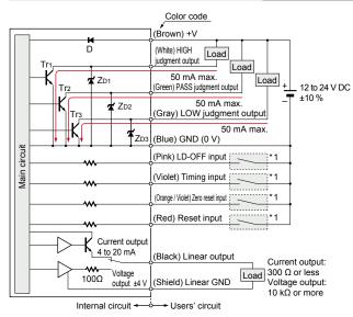
Symbols ... D: Reverse supply polarity protection diode ZD1, ZD2, ZD3: Surge absorption zener diode Tr1, Tr2, Tr3: NPN output transistor
