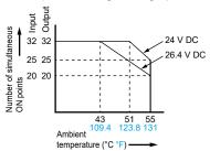
Reduce load current according to the graph below by the external power supply voltage.
