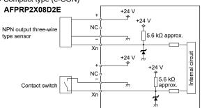
• Compact type (connector-type terminal block) [Input type]
