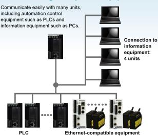
Connection to automation control equipment: 216 units (Simultaneous communication: 16 units)
