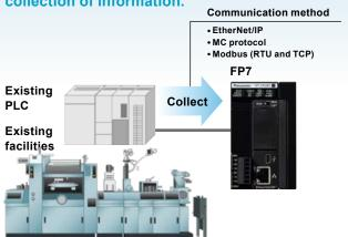
To enable information collection, because the FP7 can deal with any protocol for Ethernet / serial communications, the FP7 can be installed in existing facilities.
