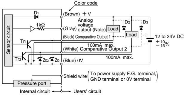
Note: When using the analog voltage output, take care to connect external equipment of proper input impedance. Also, when a cable extension is used, voltage drop due to cable resistance should be taken into account.
