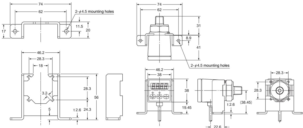
Material: Cold rolled carbon steel (SPCC)
