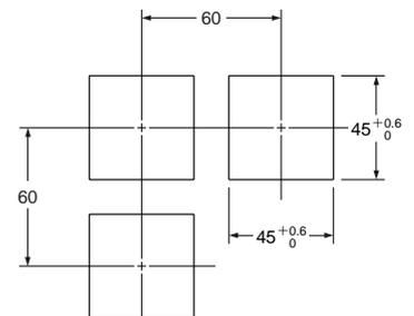
Note: The panel thickness should be 1 to 3.2mm.
