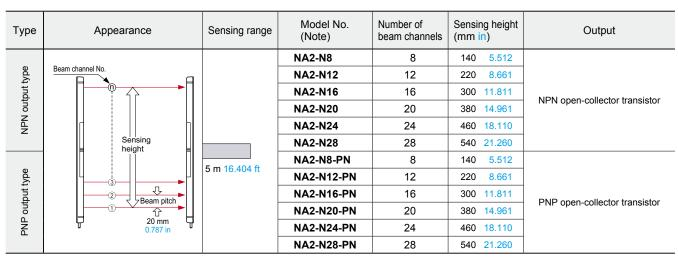
Note: The model No. with "P" shown on the label affixed to the product is the emitter, "D" shown on the label is the receiver.
