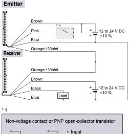
or Low: 0 to 2 V, or open High: 8 V to +V
