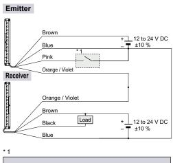
Non-voltage contact or NPN open-collector transistor
