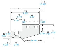
Material: Cold rolled carbon steel (SPCC) (Uni-chrome plated)
