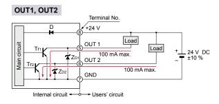
Symbols  $\dots$  D: Reverse supply polarity protection diode ZD1, ZD2: Surge absorption zener diode Tr1, Tr2: NPN output transistor
