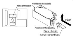
(2) Remove the battery holder from the counter.
