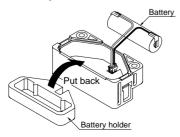
(5) Install the battery as shown below. If the cable is placed over the battery, the rear cover is difficult to fit. Hence, place the wire as shown in the figure below.
