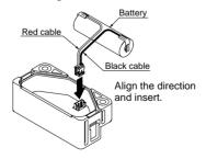
4) Put back the battery holder into the counter.
