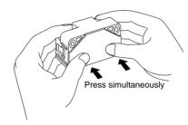
% Check that the rear cover is securely mounted. If the counter is used with improper fitting, the environmental protection is lost and the counter can get damaged.
