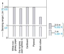
These bars indicate the sensing range with the respective objects when the distance adjuster is set to a sensing range of 2.5 m 8.202 ft / 1 m
