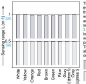
the sensing range with the respective colors when the distance adjuster is set to a sensing range of 1.281 ft.0.5 m 1.640 f long, respectively, with white non-glossy paper. The sensing range also varies depending on material.
