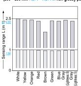
These bars indicate the sensing range with the respective colors when the distance adjuster is set to a sensing range of 2.5 m 8.202 ft / 1 m 3.281 ft long, respectively, with white non-glossy paper.
