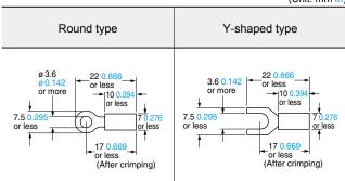
Note: Use crimp terminals with insulating sleeves.
