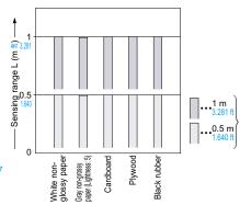
These bars indicate the sensing range with the respective objects when the distance adjuster is set to a sensing range of 1 m 3.281 ft /0.5 m 1.640 ft long, respectively, with white non-glossy
