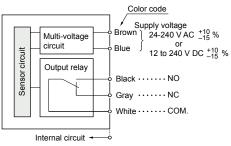
Note: The emitter of the thru-beam type sensor has two wires for power (+V and 0 V) only.
