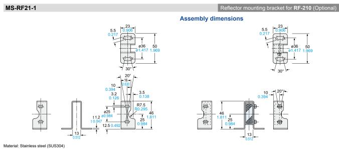
Two M3 (length 12 mm 0.472 in) screws with washers are attached.
