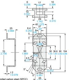
Material: Cold rolled carbon steel (SPCC) (Uni-chrome plated)
