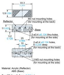
Two M3 (length 8 mm  $0.315\ \text{in})$  screws with washers and two nuts are attached.
