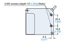
Note: Screw threads exclusive for mounting brackets. Do not use them in mounting with other products.
