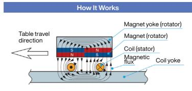
In the Nano Linear NT, the coil is subject to horizontal force due to magnetic flux constantly working vertically through the magnet and coil yoke, and rotational flux generated around the coil by the coil current (Fleming's left-hand rule). By switching the coil current direction relative to the magnetic flux direction, continuous thrust force in a single direction can be obtained, and linear motion of the rotator is maintained.
