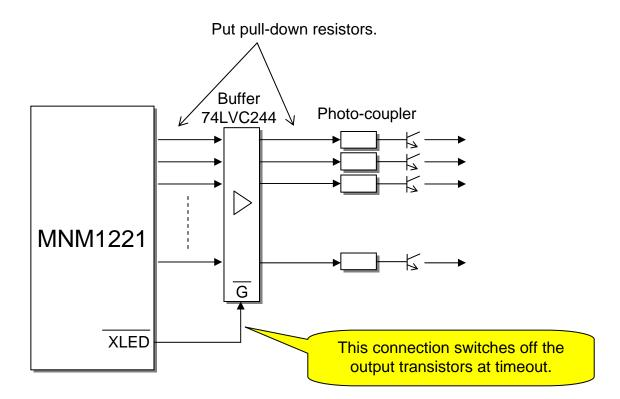
After timeout, turn off power and confirm whether communication cables has any problems.
