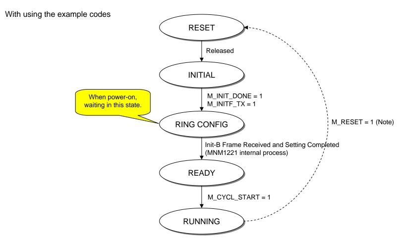
Note: If M\_RESET register is set to 1, transition can be done from any state as well as RUNNING state.
