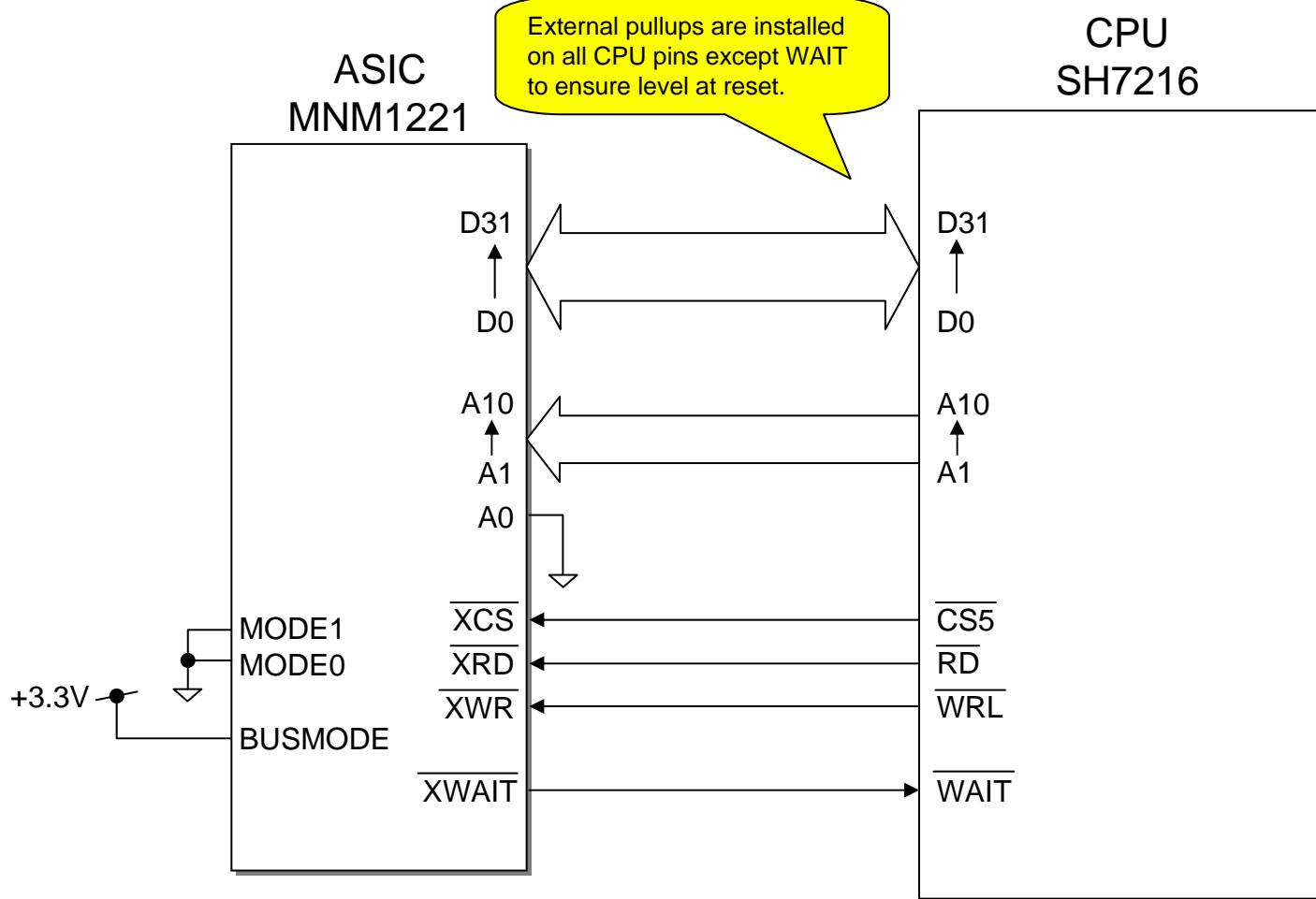
Note: A1 connection is for 16bit bus access in slave mode.
