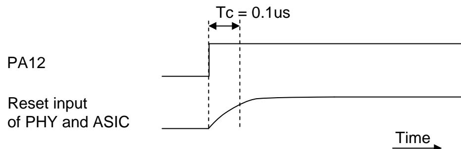
Although PA12 is Hi-Z at CPU reset, this resistor ensures low level. If watchdog timer overflows, RTEX circuit should be reset for safety. This reset causes communication timeout, and all servos will stop with timeout alarm.
