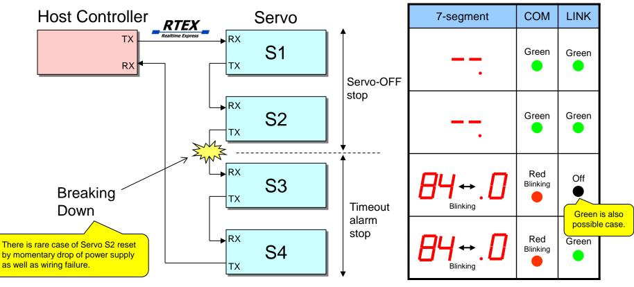
Note: 84.0 is a code that means RTEX timeout error.
