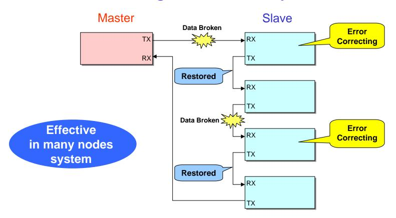
Note: Because of limitations of the error correct ability, there is a case where it cannot restore broken data.
