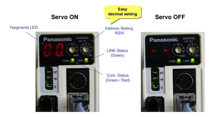
Note: If alarm, the error code is indicated on 7segments LED with blinking.
