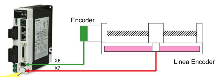
Positioning with Linear Scale
